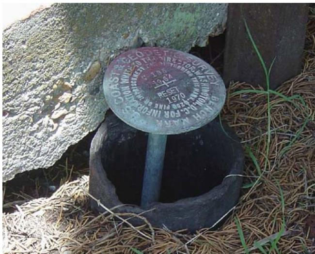
Figure 8. A Benchmark attached to a 40-foot underground rod.
