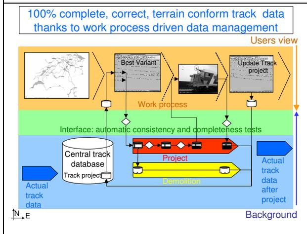
**Fig 5.** Largely automated, global track management system
