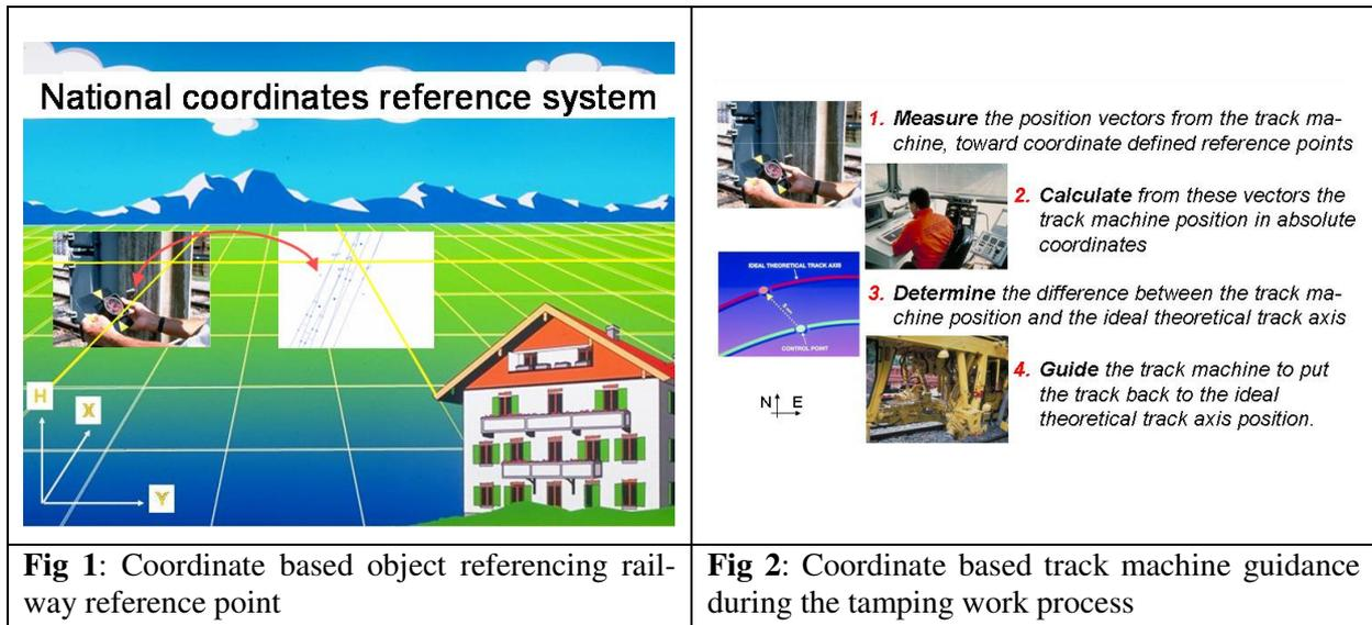
The fully automated 4 steps tamping work process steers the physical operations (Fig 2):
