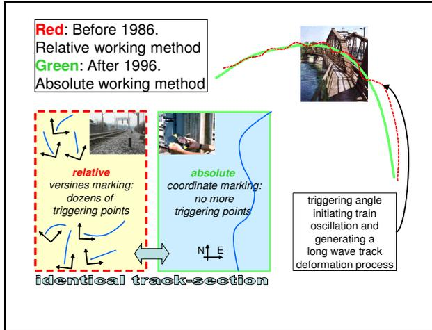
**Fig 3.** Relative versus Absolute track working methods
